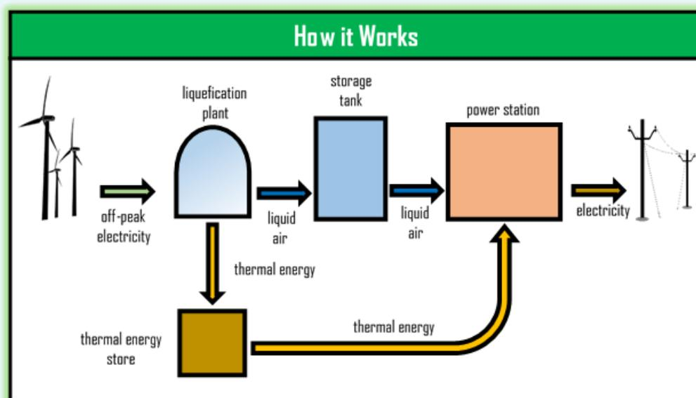
When demand for electricity increases, the stored thermal energy is used to heat the liquefied air and turn it back into a gas, and as it expands it drives a turbine to generate more electricity.
