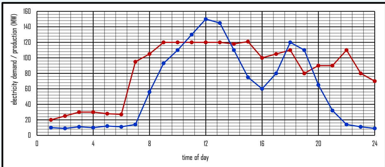
When electricity production for the wind farm is greater than electricity demand for the town the excess electricity is used to liquify air.
